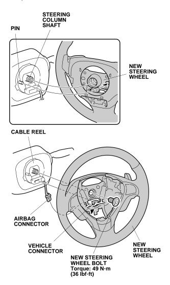
22. Install the new steering wheel bolt. Torque the new steering wheel bolt to 49 N·m (36 lbf·ft).
