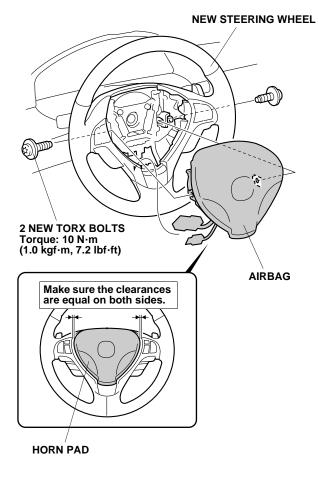
25. Reconnect the horn connector and the airbag connector. To reconnect the airbag connector, hold the pawl-side connector, and push on the back of the sleeve-side connector. Do not hold the sleeve, the sleeve is pushed back by the pawl as the two airbag connectors mate.
