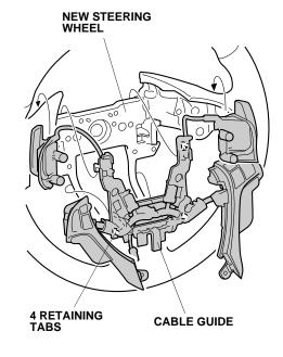
16. Install the two screws and ground terminal.
