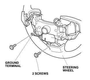
14. Remove the cable guide assembly (including both paddle switches, the audio switch, and the cruise switch) from the steering wheel (four retaining tabs).
