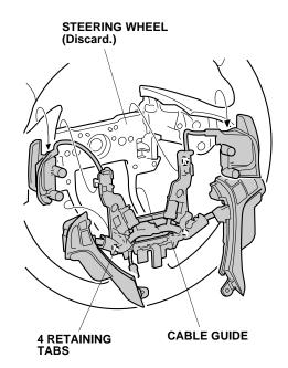
15. Install the cable guide assembly onto the new steering wheel.
